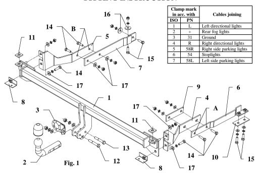
This towbar is designed to assembly in following cars: **MERCEDES 190,** produced since 10.1988 till 09.1993, catalogue no. **D04** and is prepared to tow trailers max total weight **1500 kg** and max vertical load **75 kg**.
