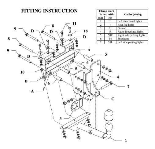
This towing hitch is designed to assembly in following cars: **OPEL ASTRA "A" ESTATE,** produced since 1991 till 2002, catalogue no. **E19** and is prepared to tow trailers max total weight **1500 kg** and max vertical mass **75 kg**.
