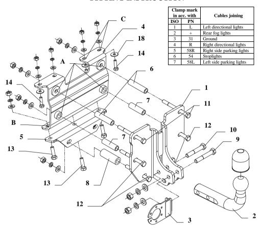
This towbar is designed to assembly in following cars: **OPEL ASTRA "A" ESTATE,** produced since 1991 till 2002, catalogue no. **E36** and is prepared to tow trailers max total weight **1500 kg** and max vertical load **50 kg**.
