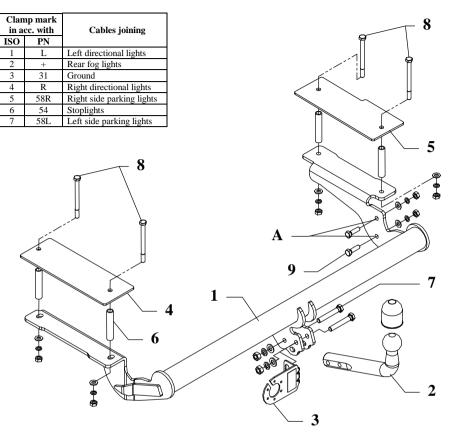
This towbar is designed to assembly in following cars: **OPEL ASTRA "B" ESTATE**, produced since 03.1998 till 2004, catalogue no. **E23** and is prepared to tow trailers max total weight **1500 kg** and max vertical load **75 kg**.
