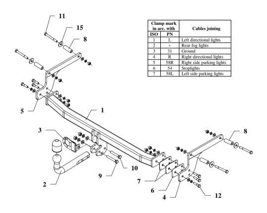
This towing hitch is designed to assembly in following car: **DACIA LOGAN, 4 doors,** produced since 2004, catalogue number **G47** and is prepared to tow trailers max total weight **1100 kg** and max vertical load **75 kg**.
